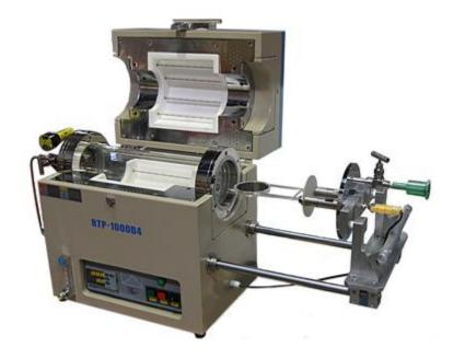
RTP-1000D4 is a compact rapid thermal processing tube furnace with 4" I.D. processing quartz tube and vacuum flange. It is designed for annealing semiconductor wafer or solar cell up to 3" diameter. RTP-1000D4 is heated by 10KW halogen light with max. 120°C/second heating rate. 50 segment precision temperature controller is built in with +/-1°C. accuracy. RS485 port and control software are included to allow you running furnace and monitoring temperature profile via PC.
