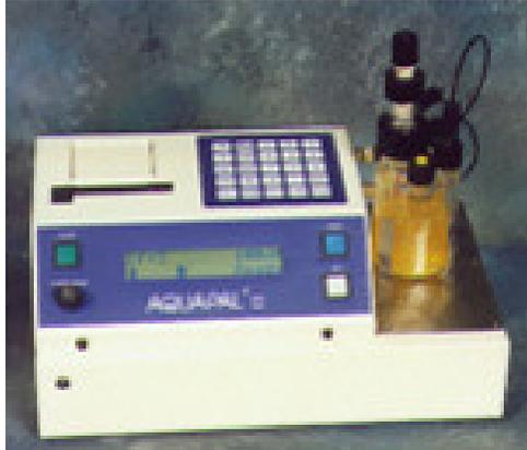
The Karl Fisher titration is a technique for the determination of moisture content developed by a chemist named Karl Fischer. It is based on a reagent which reacts with water and converts the water into a non conductive chemical.
