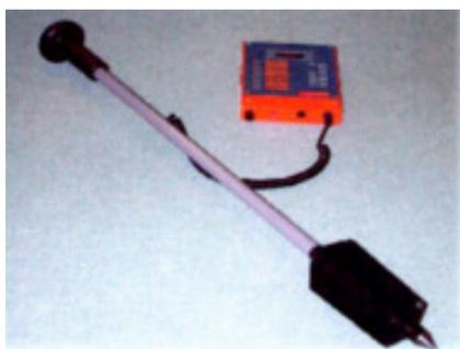
The **moisture probe** is used to penetrate into a stack, pile or holding container. The probe acts as a moisture detector at various levels in the stack of material. A single reading can be used as for quick go-no-go evaluation or readings can be taken at varying depths to get moisture profiles.
