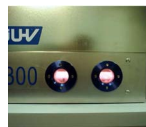
View ports at the side wall
